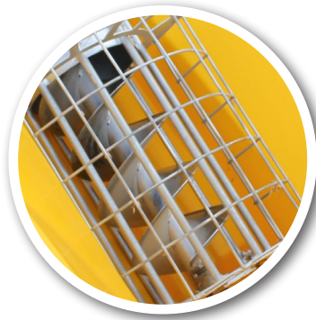
Cupped Edge Flighting Carries grain rather than dragging it.
